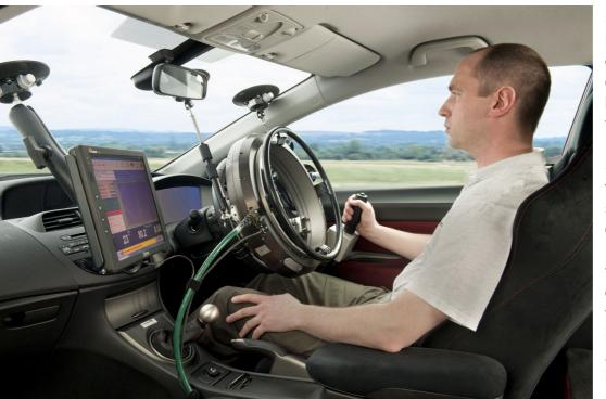
Steering robots are used for the development of vehicle dynamics, steering and braking systems, the testing of Advanced **Driver Assistance** Systems (ADAS), as well as applications such as misuse and durability testing. Using such robots for vehicle testing dramatically reduces testing time - every run is a good one. ABD robots can be installed with minimal modification to the
